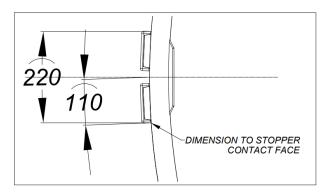
Longitudinally, stoppers need to be placed at the same distance from the leading edge as currently installed, parallel to the leading edge of the foil to align with the existing slot in the central bearing.
