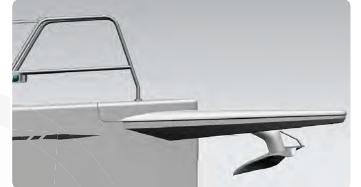
Bowsprit: New design, greater functionality for anchor and tack line
