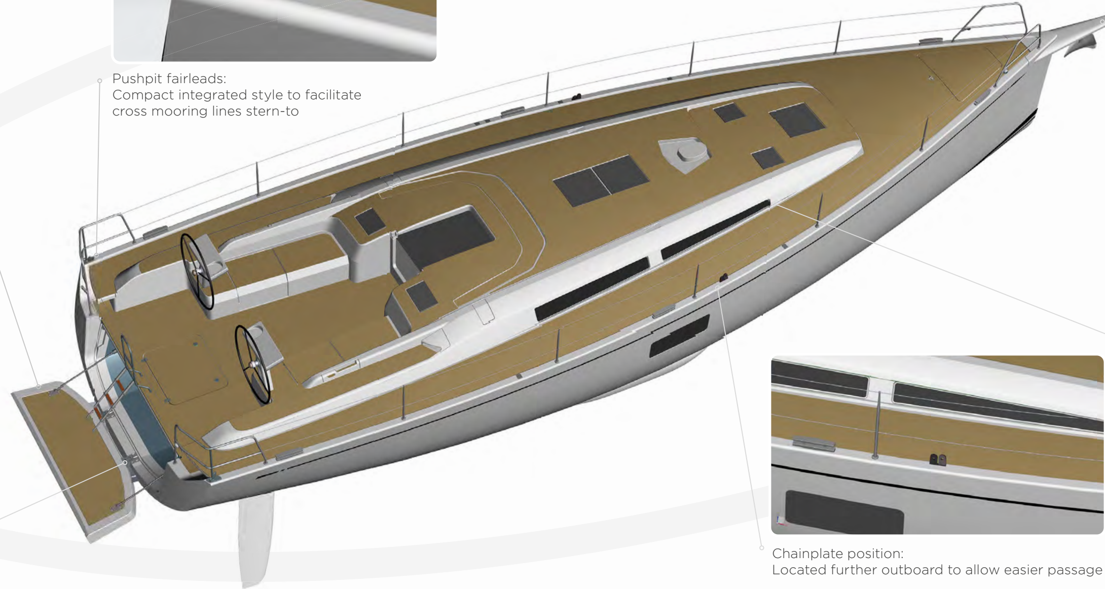
Transom door opening: New hydraulic system to enhance functionality
