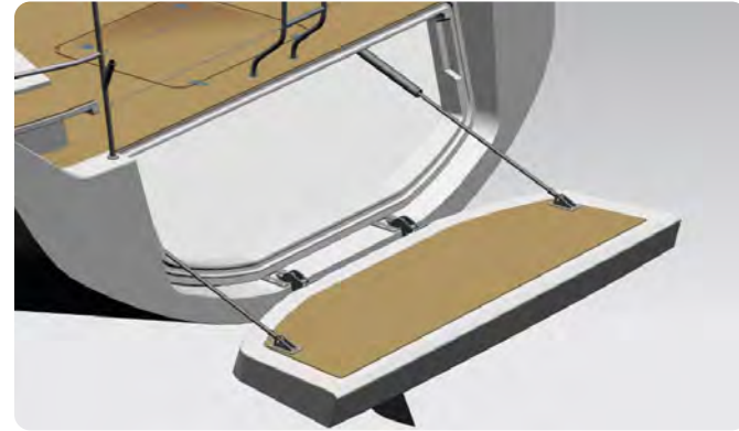
Transom door opening: New hydraulic system to enhance functionality
