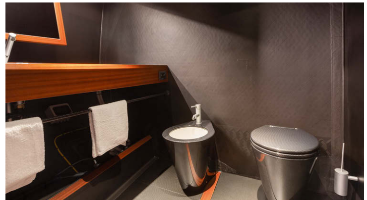
Opening pages: The ClubSwan 80 My Song sailing in the waters off the Costa Smeralda. The bow volumes are very powerful. The interiors, designed by Nauta Design, are largely removable for racing and play on the contrast between exposed carbon and mahogany trim, an essence that is a sort of style signature of the owner. The bathroom fittings are also in carbon fibre for maximum lightness; the entire 80' boat displaces less than 20 tonnes.
