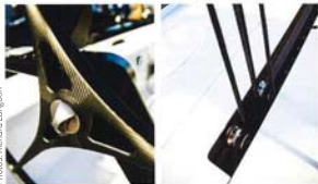
The standard of finish throughout is high. Here the mainsheet traveller is recessed below the level of the cockpit sole
