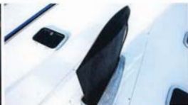
Far left: the running backstay turning blocks are covered with a fairing. Left: the centreline lifting canard has a variable angle of attack of +/- 8°
